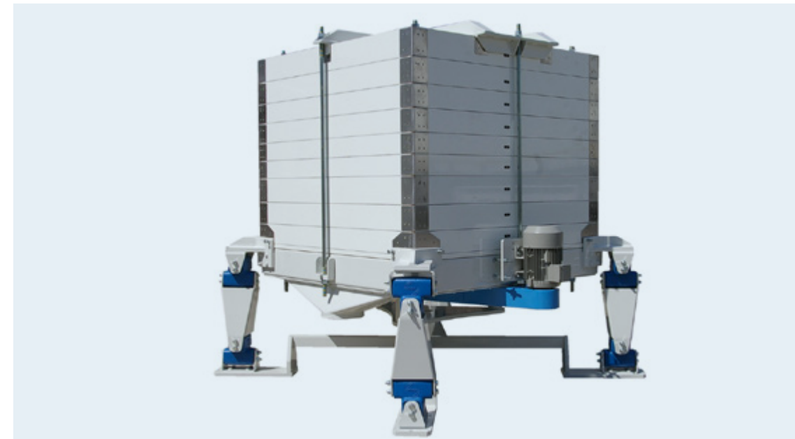
Flour Plansifter designed with ROSTA AK ®
